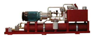
MPS starting system with all components mounted on a frame. The accumulator is mounted horizontally.
